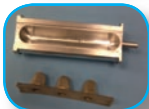
E3000-01 standard specimen holder for E3000
