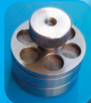
B5222 standard specimen holder for K850 (assembled)
