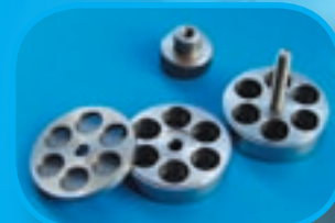
B5222 standard specimen holder for K850
