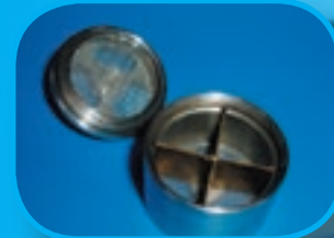
EK4150 bulk specimen holder, including divider
