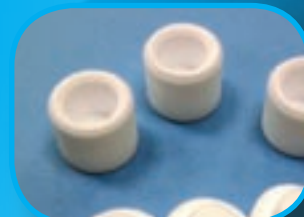
CPD800A porous pot for small or delicate specimens
